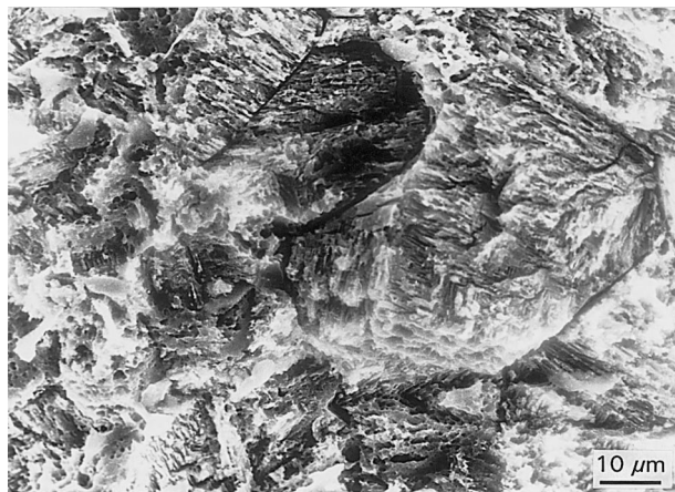
Figure 2 Scanning electron micrograph of the Ti-48Al-1V (at %) alloy after hydrogen charging for 88 h. Cracks around boundaries and intergranular cracks induced by hydrogen can be noted.
